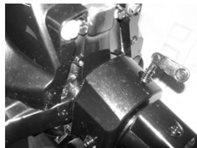
1. Cooling water checking hole
