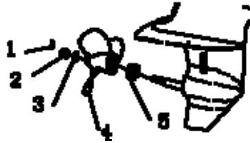
1. Cotter pin 2.Nut 3.Washer 4.Propeller 5.Thrust washer
