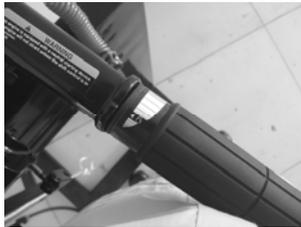
5. Pull out the choke knob fully.
