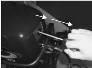
7. After the engine starts, slowly return the manual starter handle to its original position before releasing it.
