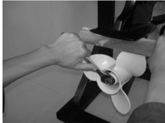
1. Check each of the propeller blades for wear, erosion from cavitation or ventilation, or other damage.
