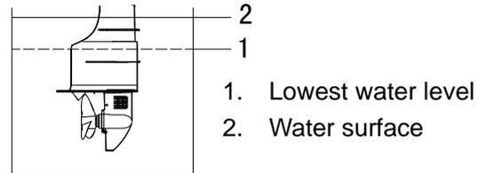
5. Fill the tank with fresh water to above the level of the anti-cavitation plate.
